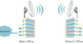
ENS500: 1-3km EnStation AC: 5-10km\* ENH1750EXT: 10-20km (with high gain directional antenna)
